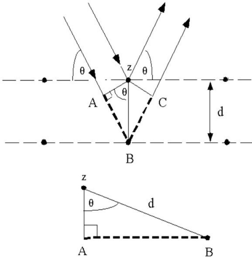
Fig. 1 Deriving Bragg's Law using the reflection geometry and applying trigonometry. The lower beam must travel the extra distance (AB + BC) to continue traveling parallel and adjacent to the top beam.
