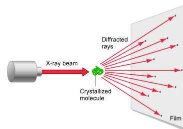
Fig 1.1 Diagram of X-ray Diffraction
